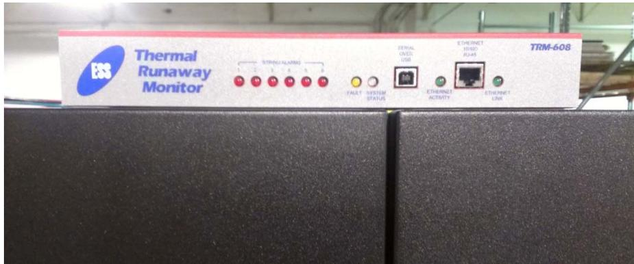
**5.1.2.** Fasten one end of the green and yellow ground cable to the back of the TRM-608 monitor and ground the unit to building. A self drilling/tapping screw is provided in the hardware kit that is included with the TRM-608 packaging. This screw can be used to screw the ground cable to a clean paint free point that is grounded to the building ground.
